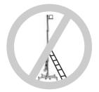
Do not lean elements (like stairs, platforms, scaffoldings, etc.) over the tower which can make pressure over it and to destabilize
