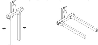
Support in stand position for transport. Extract the pin bolts and place it in horizontal position in order to locate the load.
